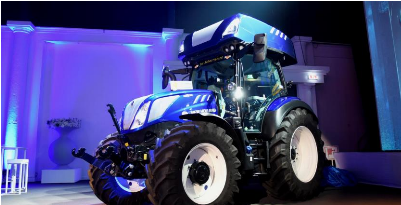
Jos Scholman/New Holland, manufacturing diesel/hydrogen dual fuel tractor, with H 2 injection in diesel engine
